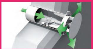
Optimum flow under inclusion of the wall conduct on the external wall is decisive for the overall efficiency of any kitchen waste air system. The flow Star wall conduct enables the combination of good flow performance, perfect seal of the wall joint with "blower door" certificate and prize-winning external appearance. Performance figures and energy efficiency may be improved even more by connection to the COMPAIR® flow flat duct system.
