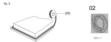
Stretch out the supplied seal along the underside edge of the hob, ensuring the ends overlap.
