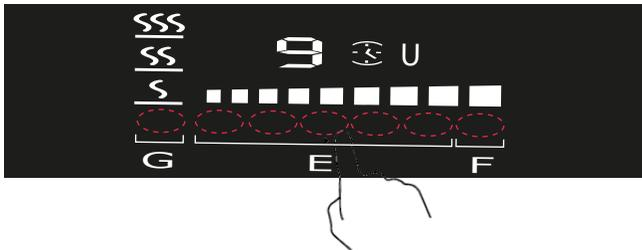
4. If the pot is moved from the front to the rear part (or viceversa),the flexible area detects automatically the new position, keeping the same power.
