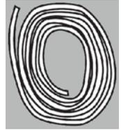
Stretch out the supplied seal along the underside edge of the hob, ensuring the ends overlap.
