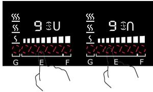
2. The flexible zone indicator **U&n** next to the power lever indicator will be light up.
