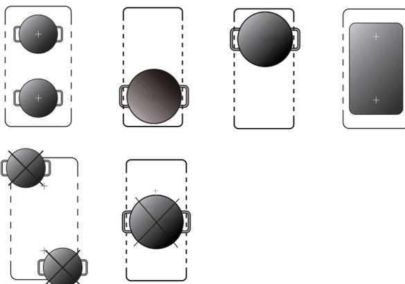
1. To activate the flexible area as a single big zone, simply press the **same time related heating zone power slider regulating key at least 2 second**
